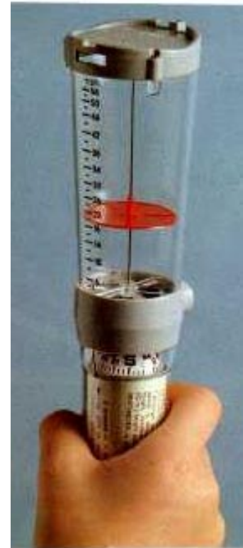
FIGURE 13 ► The ventimeter can measure wind speed and indicate wind direction
