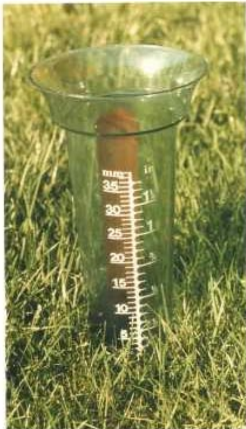
FIGURE 5 A simple plastic rain-gauge
