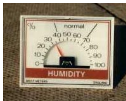
FIGURE 10 A simple paper hygrometer
