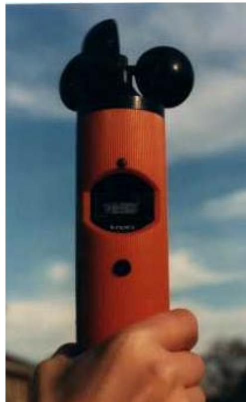
FIGURE 15 ► A simple, but accurate, cup anemometer
