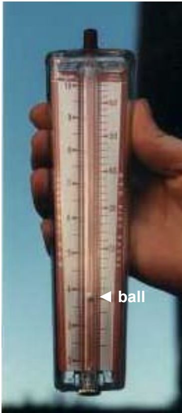
◀ FIGURE 14 The Dwyer wind-meter has a low starting speed
